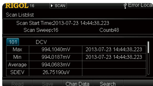
Display real-time scan information and all the measurement data of the channel selected
