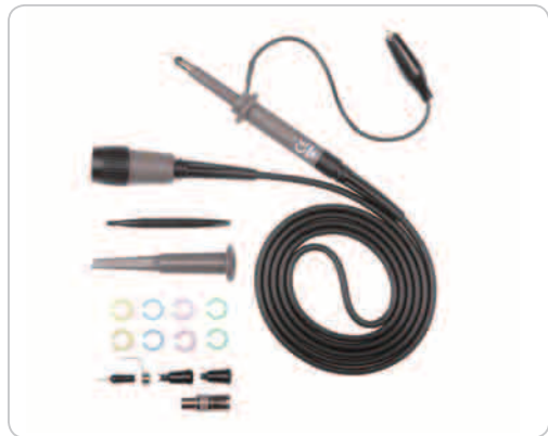
RP1300H 300MHz High Voltage Probe
