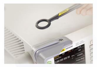
NFP-3-P3, a near-field probe which resolution is 5 mm. It is applicable for the detection magnetic field on surface. For example, the detection of the magnetic field produced by the wire, cable, metal surface, connectors, electronic components, and component joints.
