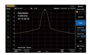
Phase noise <-80 dBc/Hz@10 kHz offset
