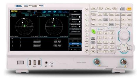
The RSA3000 series real-time spectrum analyzer includes seven models: RSA3015N, RSA3030, RSA3030-TG, RSA3030N, RSA3045, RSA3045-TG, and RSA3045N. The -TG model is equipped with the tracking generator. The frequency band range: 9 kHz to 1.5 GHz; 9 kHz to 3 GHz; 9 kHz to 4.5 GHz. The RSA3000 series has a standard configuration of GPSA and RTSA modes, capable of delivering excellent performance at low costs.
