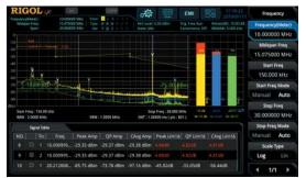
The built-in EMI pre-compliance test application software, combined with CISPR-compliant filters, makes a precompliance test on the product for conduction and radiation to identify and improve its conduction/radiation disturbance source and accelerate time-to-market.
