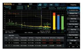
The built-in EMI pre-compliance test application software, combined with CISPR-compliant filters, makes a precompliance test on the product for conduction and radiation to identify and improve its conduction/radiation disturbance source and accelerate time-to-market.
