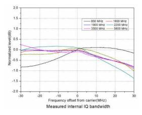
Support internal and external IQ modulation
