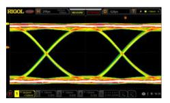
After you have purchased the DS70000-JITTA option, the DS70000 series supports the eye measurement for all the analog channels, and also provides measurement for several parameters of the eye diagram: eye height, eye width, eye amplitude, crossing percentage, and Q Factor. It also supports various clock recovery methods, such as Constant (automatic, semi-automatic, and manual), Firstorder PLL, Second-order PLL, and Explicit, to meet the demands of customers for different application scenarios.
