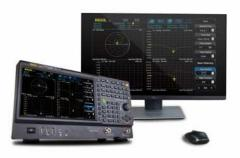
The instrument can be connected to a larger display/ monitor via the HDMI interface for better display effects. The Web Control function allows you to directly control the device by accessing the device IP address, improving remote control user experience.
