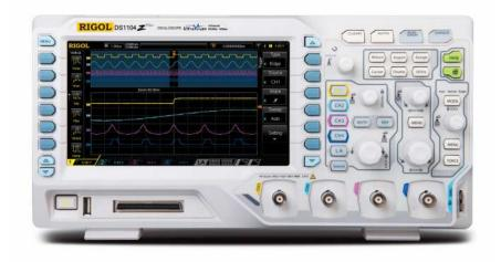
DS1000Z series is the high performance, economic level general purpose oscilloscope which provides 4 analog channels, 4 bandwidth models (50 MHz, 70 MHz, 100 MHz, and 200 MHz), and up to 1GSa/s sample rate. With the UltraVision technical platform, the DS1000Z series has sustained its deep memory and high capture rate, exhibiting its cost-effective advantages.
