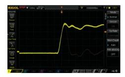
UltraVision: waveform capture rate up to 30,000 wfms/s
