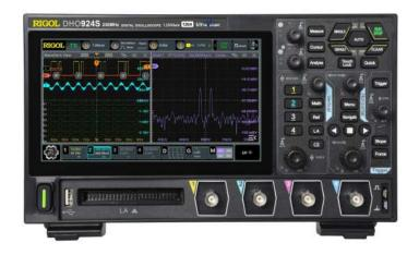
DHO900 series is RIGOL's new launched high-performance economical digital oscilloscope. Compact in size, the DHO900 series features a capture rate up to 1,000,000 wfms/s (in UltraAcquire Mode), 50 Mpts, 12 bits resolution, and low noise.
