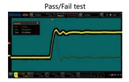
The MSO7000/DS7000 series is equipped with hardware pass/fail test function as the standard configuration, which can be used in signal monitoring for a long time, signal monitoring during design, and signal test in the production line.
