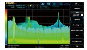
The RSA5000 series delivers up to 40 MHz of real-time bandwidth using the innovative Ultra Real technology. In the real-time bandwidth range, transient signals exceeding 7.45  $\mu$ s duration can be guaranteed to be 100% captured and accurately measured.
