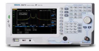
With a compact size and light weight, the DSA700 series spectrum analyzer has an excellent technical specification. Its measurement frequency range is from 100 kHz to 1 GHz. The high cost-effective spectrum analyzer with a high performance makes it popular with the users.
