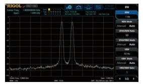
DANL low as -161 dBm effectively ensures the testing for the weak signals, reducing the impact of the noise floor of the spectrum analyzer.
