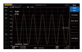
Zero span to demodulate the AM signal
