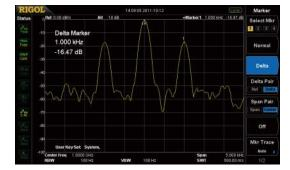
Provide a high RBW of 10 Hz to identify signals with similar frequencies
