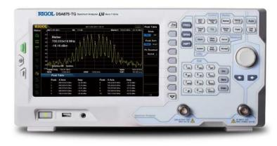
With light weight and compact size, the DSA875, DSA832/E, and DSA815 series spectrum analyzer has excellent technical specifications. Their frequency bands can reach 7.5 GHz, 3.2 GHz, and 1.5 GHz. DSA815 is an entry-level spectrum analyzer, with its frequency range of 9 kHz to 1.5 GHz. It is an economical instrument with an affordable price.
