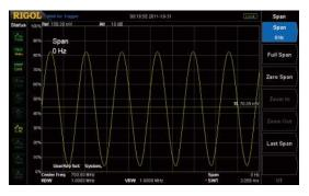
Zero span to demodulate the AM signal
