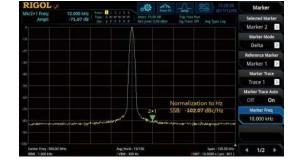
Excellent sweep specifications; phase noise low as -102 dBc/Hz.
