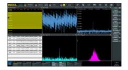
It has a delicate industry design, and it is a 7U full-rack structure that includes two touch screens. The main display is a 15.6-inch capacitive high definition touch screen with one button electronic tilt. Multi-pane windowing supports a variety of simultaneous analysis tools, making it easier to view signals, measurements, and results. Meanwhile, the secondary 3.5-inch touch screen separates menus and functions from signals and analysis with a customized function and shortcut menu.
