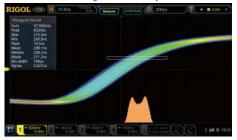
The histogram enables users to observe the measurement results of signal variation in a long period of time, helping them locate the potential abnormalities of the signal.
