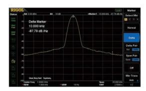
Phase noise <-98 dBc/Hz@10 kHz offset (DSA832/875)
