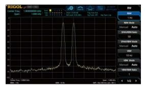
Resolving signals with similar frequencies is critical to verifying many RF devices and systems. With the RSA3000, the 1 Hz RBW allows you to view more details of adjacent signals.
