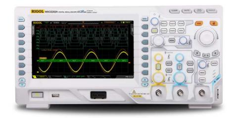
MSO/DS2000A series provides bandwidth from 100 MHz to 300 MHz, sample rate up to 2 GSa/s, and 2+16 channels. It is easy to operate. With a variety of functions, the user-friendly UI design, and the 256-level intensity grading display that allows you to see the signal anomalies clearly, it is a helpful tool in addressing the challenge in application scenarios such as circuit design, embedded debugging and power supply design.
